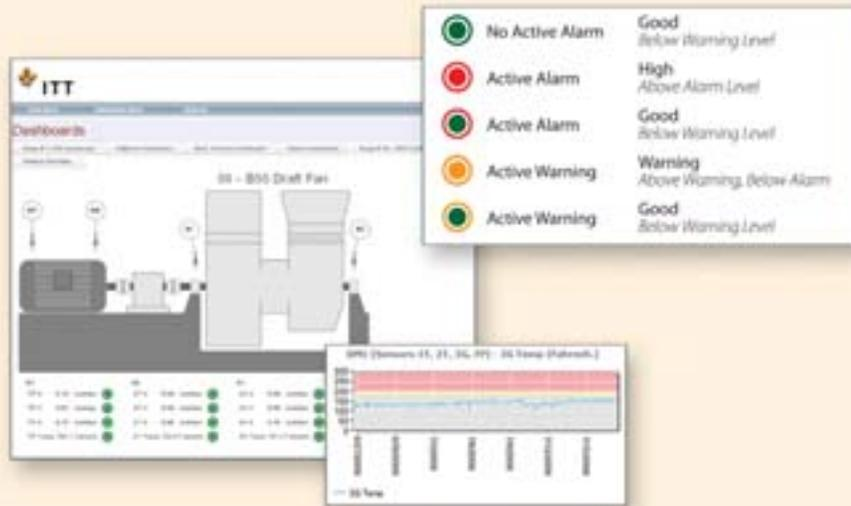
Dashboards take the abstract nature of your machine data and ties it into a visual representation of your machine. ProNet uses easy-to-understand status circles to quickly identify the condition of each machine. A rollover 'quick-view' plot of critical data can be viewed from the Dashboard.
